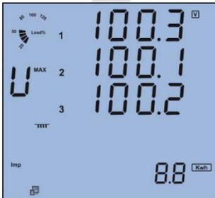
Fig 3.25 Max phase voltage
