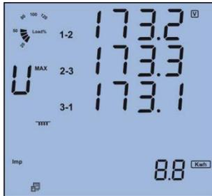
The second screen: Max value of the line to line voltage.
