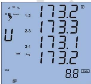
Fig 3.4 Three phase to phase voltage
