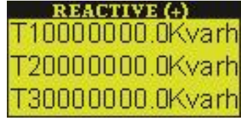
Figure 34 import reactive energy window1
