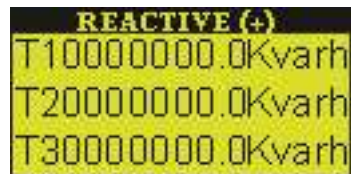
Figure 34 import reactive energy window1
