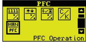
Figure 48 PFC Operation is MANUAL
