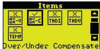
Figure 65 Over/Under Compensate is enable
