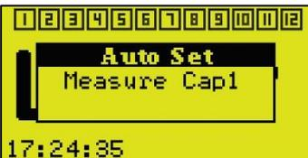
Figure 7 Turn on Capacitor1
