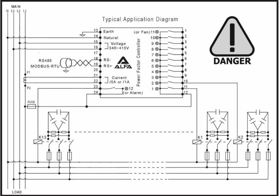
Figure 2 Wiring diagram
