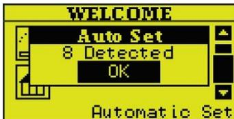
Figure 116 Automatic Set Shows Number of Detected Capacitor Steps
