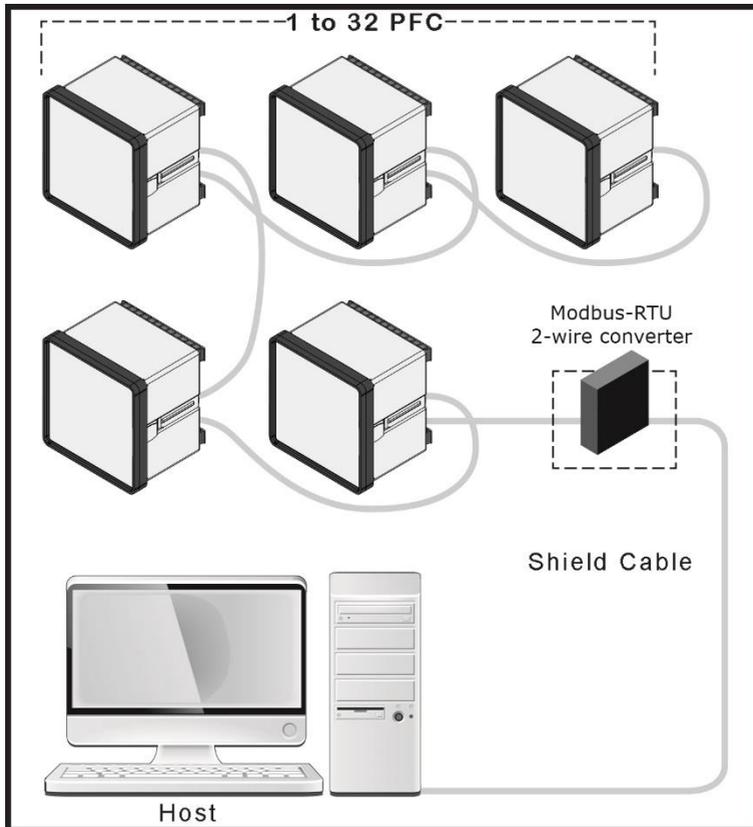
Figure 123 communication wiring
